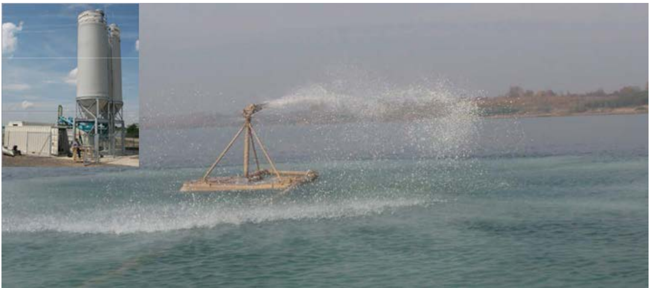
Fig. 6: Upper left: Lake Hain stationary neutralisation plant and its floating unit for above water distribution (source: UIT/LMBV)
