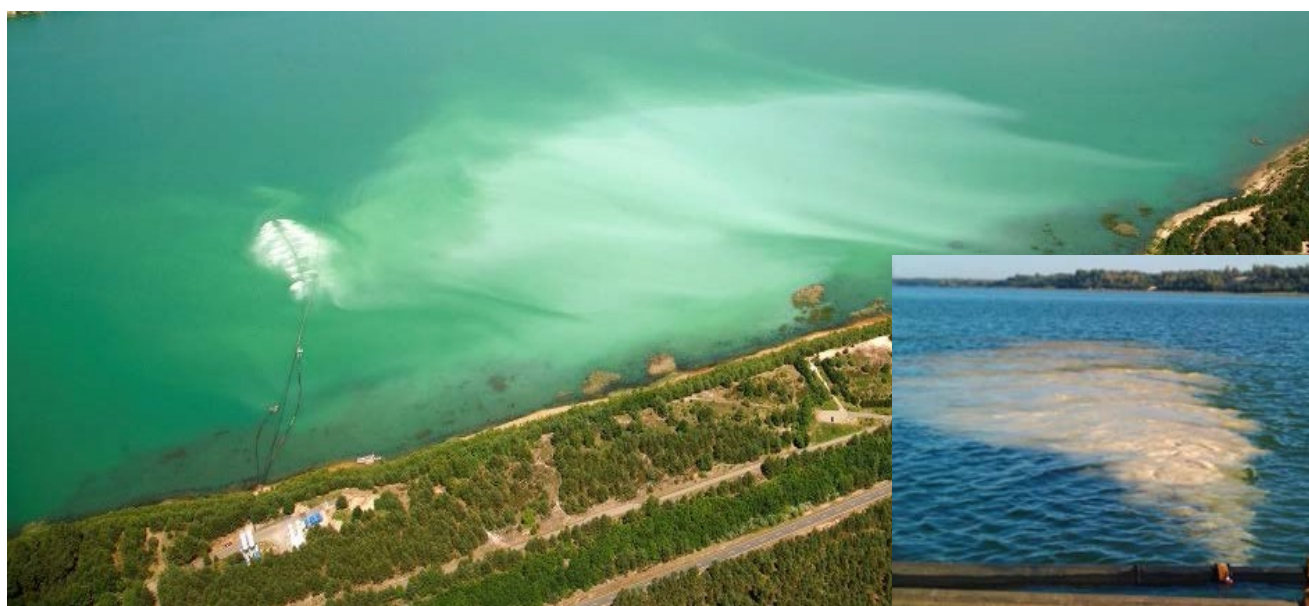
Fig. 16: GSD plant on Lake Scheibe with a submerged input system (close-up) and distribution of the lime suspension in the lake (source: GMB)
