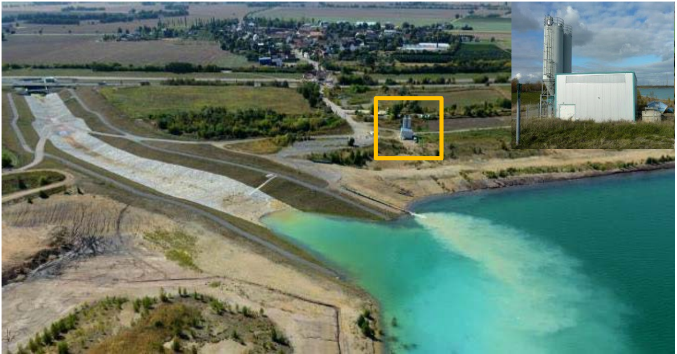
Fig. 15: Stationary neutralisation plant on Lake Zwenkau and the lime plume spreading in the flooding water (source: LMBV)
