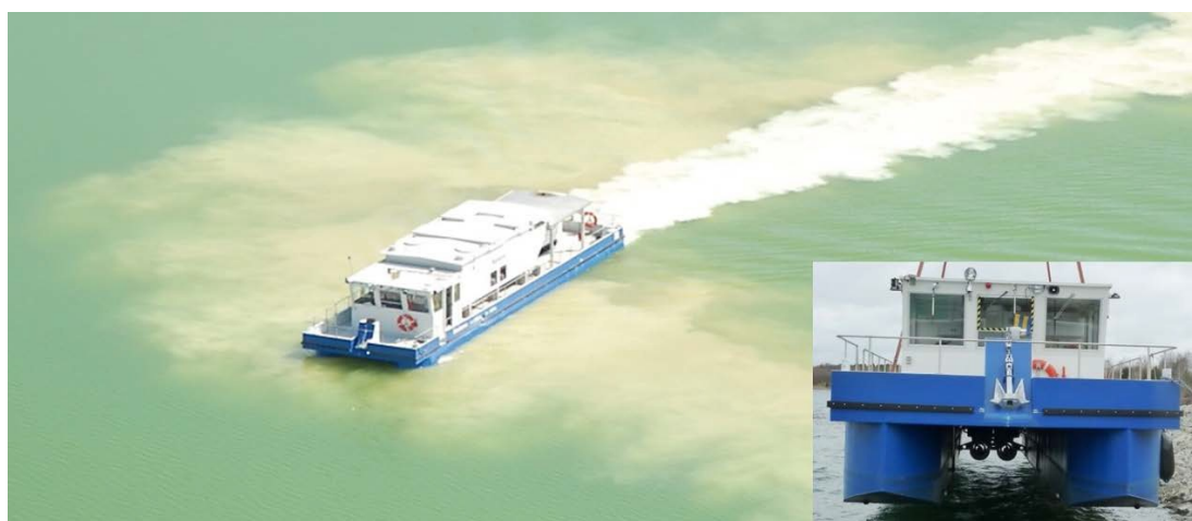
Fig. 11: Water treatment vessel Barbara in operation, and (bottom right) being lowered – showing the delivery system between the vessel's hulls (source: LUG/LMBV)
