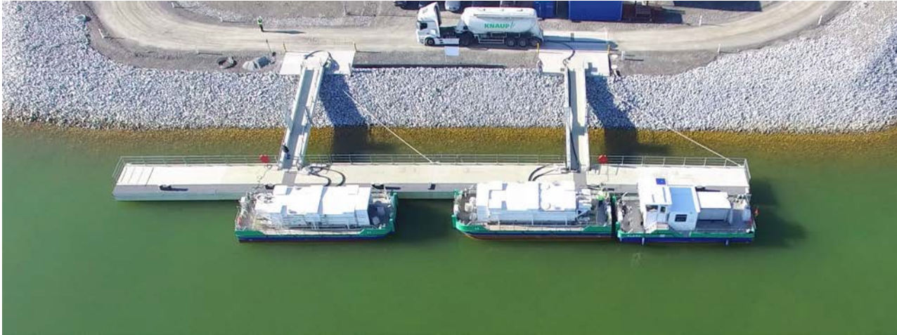
Fig. 14: LMBV water treatment vessel Klara coupled to Lighter 1 (right), and Lighter 2 (left) at the landing and loading site (source: [33])
